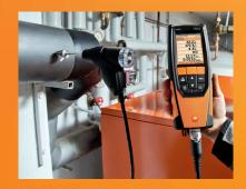
To pair the combustion analyzer to your smart device, turn on the testo 320 with Bluetooth, and run the testo Combustion app. Once the app is running, select the correct serial number in the App, and the device will pair automatically.
